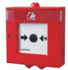
For immediate manual actuation of a fire alarm. Direct alarm actuation by pushing in the glass plate. By replacing the glass plate the push button is reset and the device is ready for operation again.
