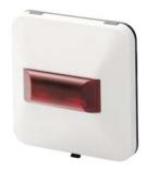
The alarm indicator is connected in parallel to automatic fire detectors in order to indicate quickly the source of an alarm signal from detectors that are not easily accessible or visible. The alarm indicator contains an indicator lamp unit with one or two LEDs. They light up as soon as a connected fire detector gives an alarm.
