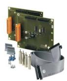
The connector board is necessary if the operating add-on (2xEVAC) is used remote from the control panel in a separate housing. The connection to the control panel occurs via the RS485 interface. The remote access to the operating add-on is possible until 1000 m.
