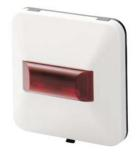
The alarm indicator is connected in parallel to automatic fire detectors in order to indicate quickly the source of an alarm signal from detectors that are not easily accessible or visible. The alarm indicator contains an indicator lamp unit with one or two LEDs. They light up as soon as a connected fire detector gives an alarm.
