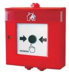
For immediate manual actuation of a fire alarm. Indirect alarm actuation by pushing in the glass plate and pressing the push button. To replace the glass plate, open the housing door with the key. The push button must be reset before closing the door again.
