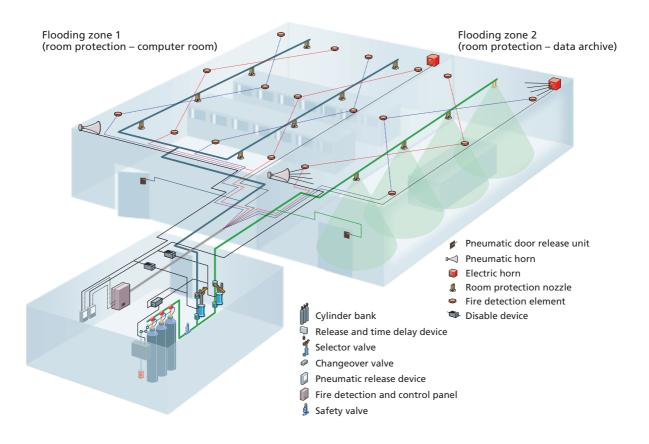
Supply of extinguishant in low-pressure vessels If large quantities of extinguishant are needed for the overall safety concept, a low-pressure vessel is recommended – especially on grounds of economy.
